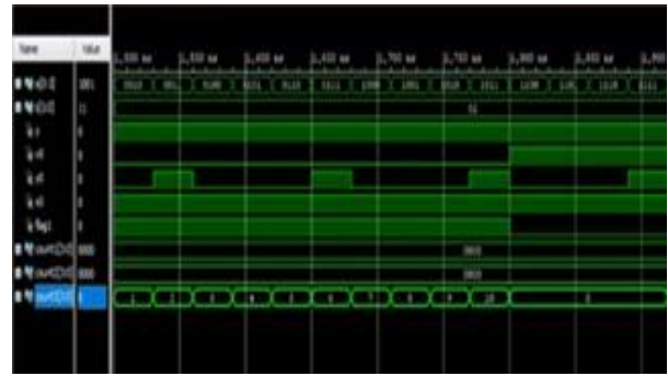
Fig 6: Simulation result for stuck – at – one fault
